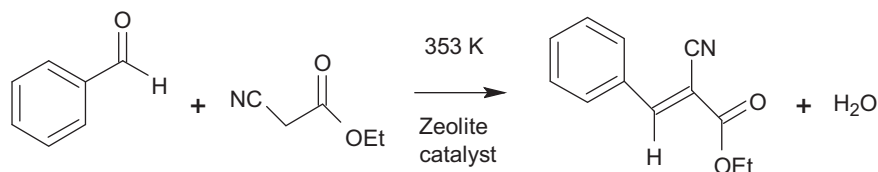
Scheme 1. The Knoevenagel condensation between benzaldehyde and ethyl cyanoacetate.
